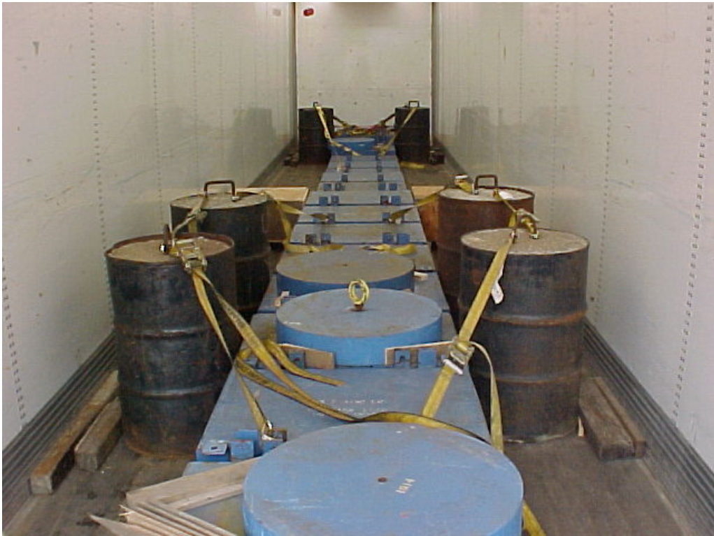
Figure 2-2 Trailer Payload giving 49,400 kg GW
